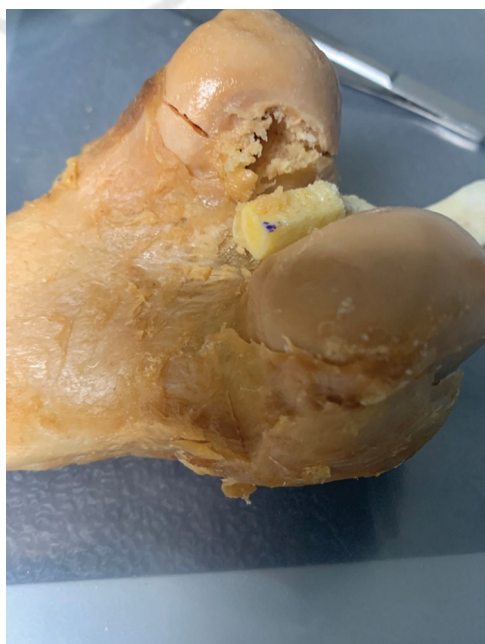
Fig. 3 Group 1 patellar plug fixated with condylar fracture at peak tension load to failure.
