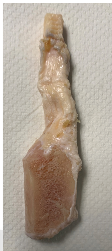
Fig. 4 Group 6 tibial 10 mm bone plug post tension load to failure demonstrating entire length of bone block was pulled out of the socket without fracture. Also, demonstrating zero divergence of screw based on uniform screw threads throughout the entirety of the tibia 10 mm bone plug (top). Patella side untrimmed.
